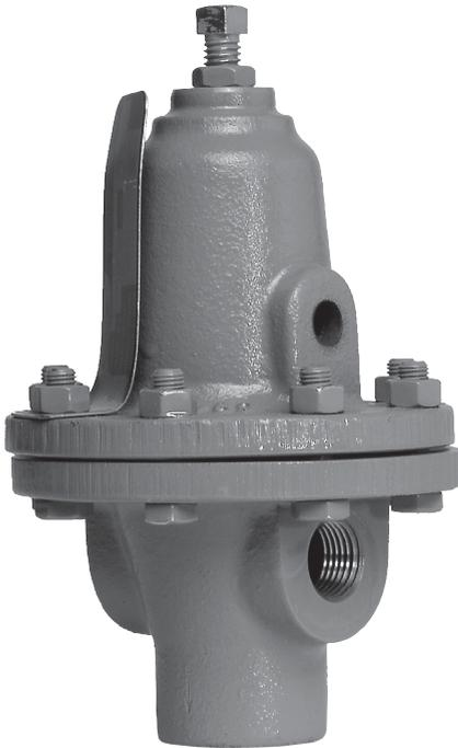
The Model BQ Back Pressure Regulating Valve is a self-operated, spring-loaded back pressure regulating valve. Typically the Model BQ is installed at the far end of the oil supply line, downstream of the boiler fuel metering valves and passes unburned oil to the return line. Alternately, the Model BQ may be installed upstream of the boiler fuel metering valves. In both cases, the valve passes oil to the return line in order to maintain a constant supply pressure to the fuel metering valves.
